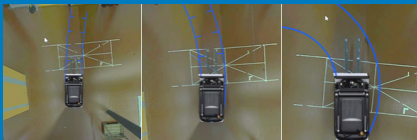
Automatic zoom function to simplify low-speed manoeuvring in narrow environment
