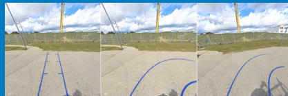
Digital panning of camera depending on the steering angle allows the driver to see more of the relevant area
