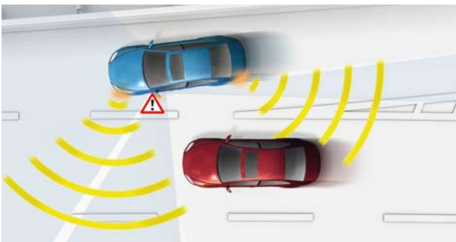
Side View Assist reduces the risk of accident during lane changes by warning the driver
